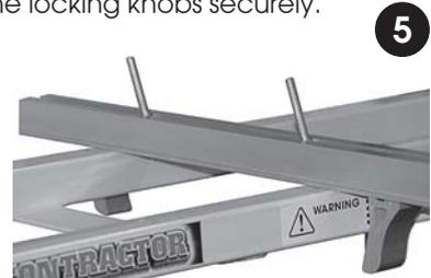
**NOTE:** Should the tool not have suitable holes for mounting to the table, then the tool should firstly be mounted on to a suitable board of at least 15mm thickness, and the board, with tool, secured to the table, again using the carriage bolt provided.
