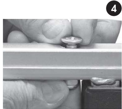
2. Attach the stabilisers, one to each leg, as shown in Figs 3 and 4.
