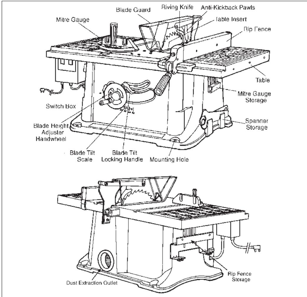
1. The switch panel incorporates the ON and OFF switches.
