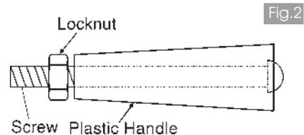
When properly assembled, the handle will rotate freely about the screw, with only a small amount of end play.
