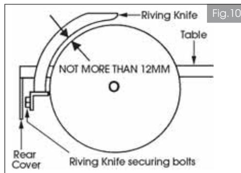
Should the Riving Knife subsequently become out of shape or misaligned, it must be gently eased back into line, or if the damage is more severe, it must be removed and bent back into shape accordingly or replaced.
