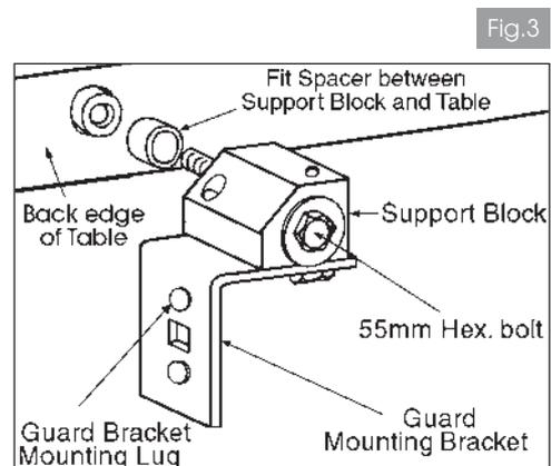
3. Thread the 55mm bolt through the hole in the NON RECESSED end of the Support Block. (see fig 3), with the lock washer, followed by the flat washer up against the bolt head.
