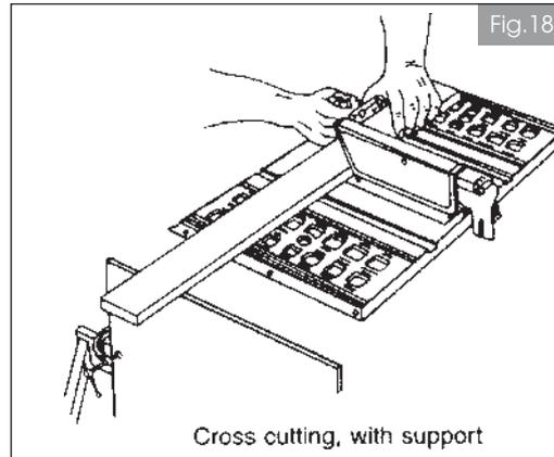
For maximum accuracy when using the mitre gauge, always favour one side of the groove in the table. In other words, don't move the mitre gauge from side to side while cutting but keep one side of the bar riding against one side of the groove.
