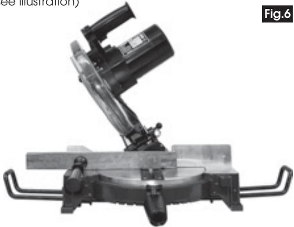
The 45° adjuster is factory set so that when the Head is tilted to its fullest extent the blade will cut 45° bevel.
