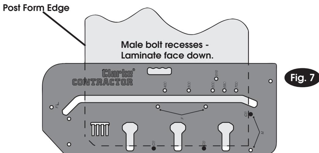
24. Place the router into the front of one of the clamp bolt recesses, set the depth of cut to 10mm max. Switch the router ON and machine the recess. When done, switch the router OFF and wait for the cutter to stop spinning. Return the router to the back again. Increase the depth of cut a further 10mm and machine the recess again. When finished, switch the router OFF and wait for it to stop spinning.
