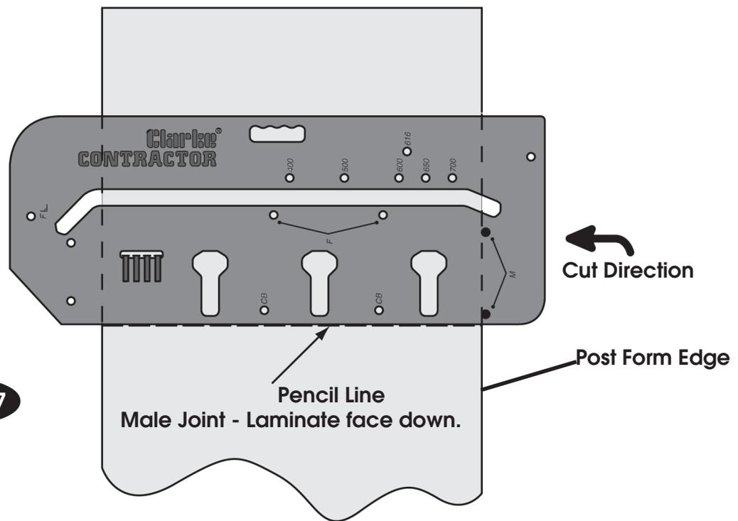
11. Firmly clamp the jig to the worktop ensuring it doesn't move as you do so. Ensure the clamps do not obstruct the router path.
