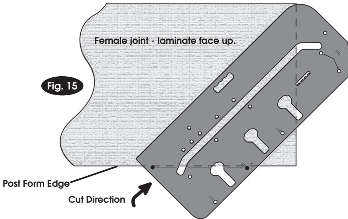
4. Ensure the 2 pins in holes 'F' are pushed firmly against the post form edge of the worktop, clamp the jig to the worktop ensuring clamps do not obstruct the router path.
