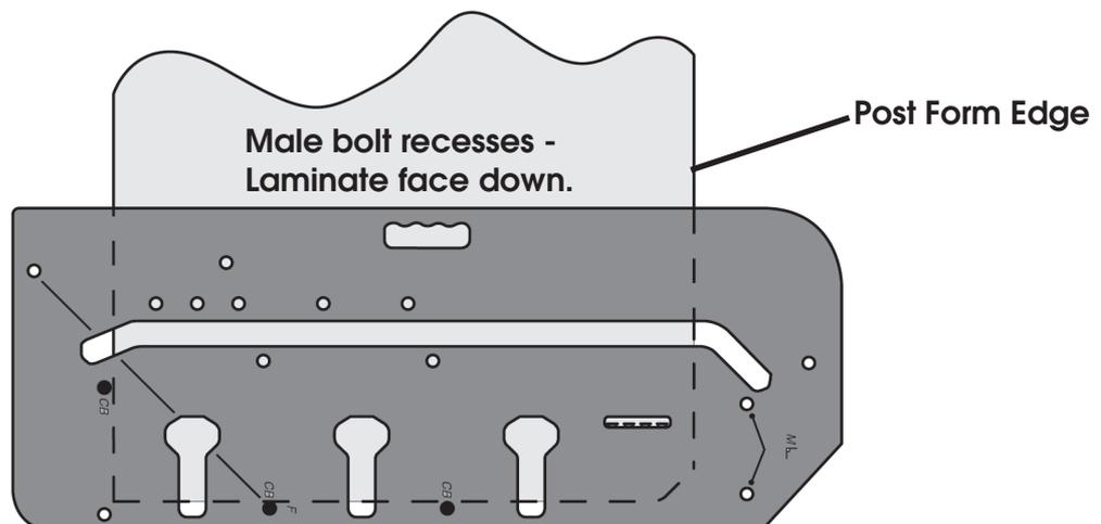
19. Fully insert 3 pins in the holes marked 'CB'.
