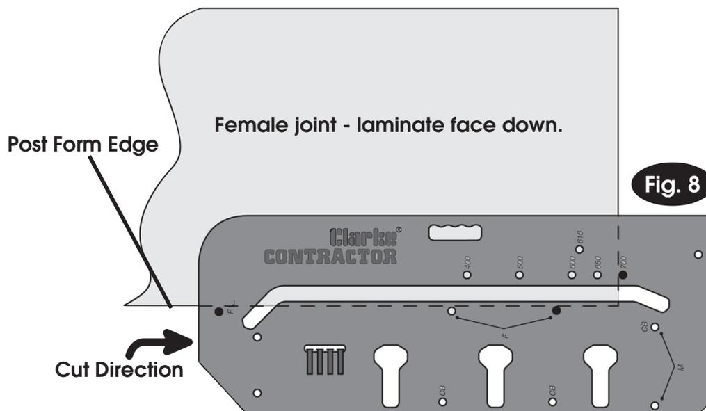
5. Firmly clamp the jig onto the worktop ensuring the clamps do not obstruct the router path.
