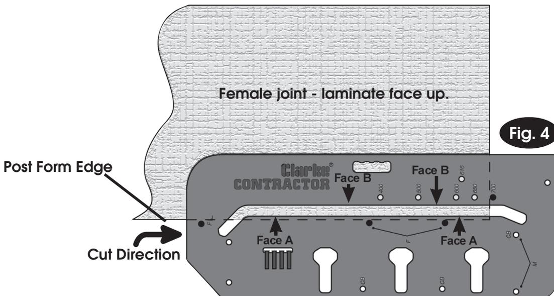
4. Ensure the 3 pins in holes 'F' are pushed firmly against the post formed edge, and the fourth pin in the hole marked with the worktop width is pushed firmly against the worktop edge.
