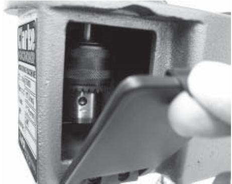
10. Insert the drill bit into the chisel then insert the chisel and bit up through the hole in the head.
