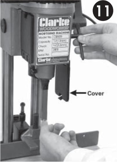
11. Push the drill bit up through chisel, and into the opened jaws of the chuck as far as it will go, then back off approx. 1/16" (2mm). Secure the drill bit in this position, by tightening the jaws using the chuck key provided.
