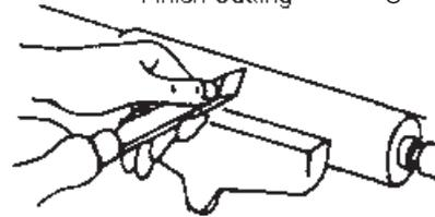
Finish cutting requires more control with less force and is better done with the palm of the tool rest hand turned up. The wrist is still held down, and the side of the index finger acts as a guide along the rest. In this position, control of the chisel is shared by both hands, the fingers of the tool rest hand being free to assist in positioning the tool.
