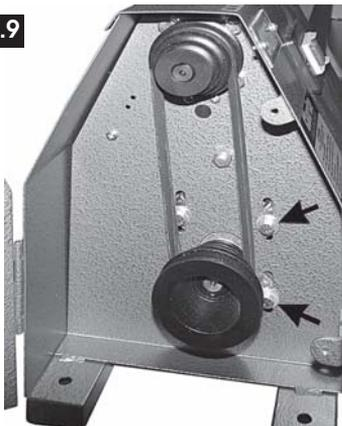
Fig.9 shows the belt positioned on the second step from the outside face of the pulley. This produces a spindle speed of 1750 RPM. (Refer to the chart above).
