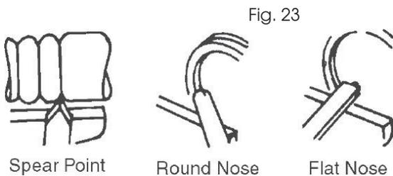
A 1/2" wide spear point chisel, a 1/2" wide round nose chisel and a 1" wide flat nose chisel complete the list of tools ordinarily used by home craftsmen. Each of these scraping chisels can be purchased in various other sizes for special purposes. All are very useful for diameter scraping operations and for circumference
