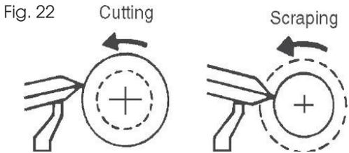
The parting tool has just one primary purpose to cut straight into the workpiece as deep as desired, or all the way through to make a cut-off, it is therefore a very narrow tool. 1/8 inch wide and shaped to cut its own clearance so that the edge will not be burned. When used for scraping, however, it should be backed off regularly to prevent overheating.
