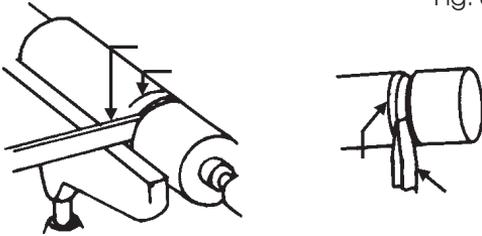
First, mark position of the shoulder with a pencil held to the revolving workpiece. Then make a sizing cut with the parting tool, placing this cut about 2mm outside the shoulder position and cutting to within about 3mm of the depth desired for the area outside of the shoulder.
