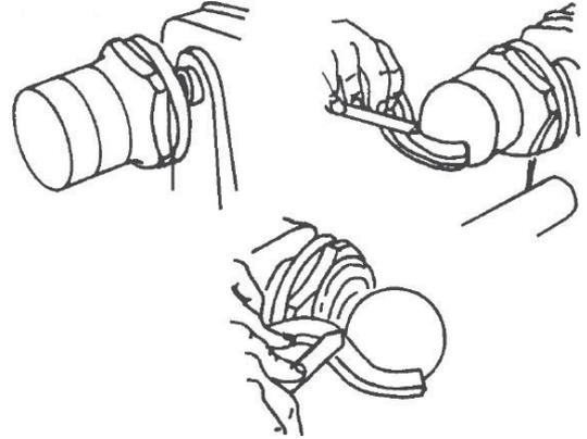
Wooden balls of large size are first roughly turned between centres, using standard procedures. Smaller balls can be mounted as face plates on the small faceplate of screw centre. Lines drawn to indicate the centre and ends of the ball shape are helpful in plotting the curve. A template should always be used for accurate visual observation of the work progress.
