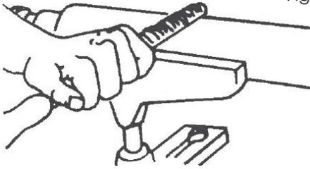
A wood rasp will remove stock quickly when held against the revolving workpiece. Care should be taken to support the rasp firmly against the tool rest however, as it can tear the hands painfully if caught by a rough edge of the workpiece and kicked back. The rasp will leave a very rough finish.
