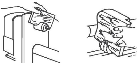
The drum is used mainly for sanding the edges of curved work. The squareness of the edge of the work can be best retained by using a simple form of vertical fence as shown. The standard sanding drums are commonly made with a threaded hole to fit the Lathe Drive Spindle. To guard against loosening of the taper shank while the drum is in operation, it is advisable to support the free end, using either a ball bearing or plain 60° centre in the tailstock.
