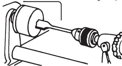
Proper support must be provided at all times for the scraping chisels. Several tool rest positions are shown in the accompanying illustrations. Always endeavour to position the part of the rest that supports the tool as close to the working surface as possible.
