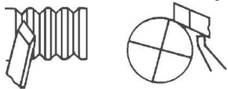
When the heel is used, the skew is rotated down into the work, using the rest as a pivot. Otherwise, the cutting position and sequence of cuts is the same.
