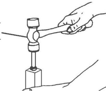
Drive the centre into the wood. Use a wooden mallet or a plastic hammer, but put a piece of wood on the end of the centre to protect it.
