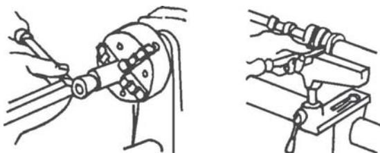
Standard wood turning chisels are excellent for turning plastics by means of scraping methods. The tool rest should be slightly below centre and the chisel handle should be held a little higher than the cutting edge to give a negative rake. Scraping tools should be kept to a minimum. A large contact area, such as the full edge of the spear-point chisel, will cause chatter and probable chipping.
