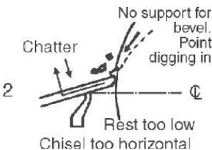
chisel, then the improperly supported chisel will begin to bounce, or chatter, against the workpiece.
