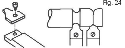
An old chisel can be made to serve as a holder for 'shaper' or 'moulding' knives. Such knives make it possible to scrape many interesting shapes in the workpiece surface in one or two operations instead of the many operations required with standard chisels. It is generally not practical to use cutting methods with special shape tools, scraping methods should be used.
