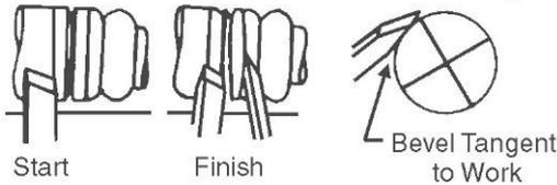
It is important that only the extreme heel should do the cutting. This means that the bottom edge of the bevel, next to the vee, must at all times be tangent to the arc of the bead being formed.
