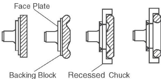
After being chucked the remaining face of the ring can be turned to the proper contour, thus cutting away the centre portion.
