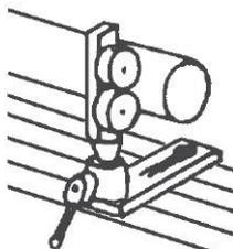
Position the backstick against a pre-turned portion near the centre of the spindle, this portion being at least 3mm over finish size to allow for later removal of any marks made upon it.
