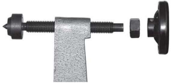
4. Disassemble the Tool Support Bracket, and reassemble to the machine in the manner shown in Fig.6. The Clamping Bracket and Lever should be oriented in the same manner as for the Tailstock.
