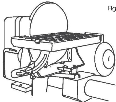
The sanding disc is a metal plate with a threaded shank which fits the end of the lathe spindle. Abrasive paper is glued to the machined surface of the plate by means of a quick drying cement supplied for this purpose. Abrasive discs can be purchased or cut from the standard sizes of abrasive paper.
