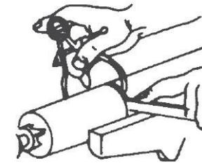
The roughing-off cut can be made to accurately size the cylinder to a given diameter.
