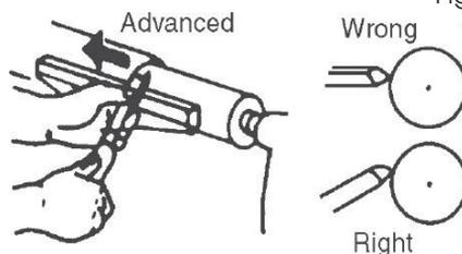
Three gouges the 1/4", 1/2", and 3/4" are ample for general DIY turning, but other sizes from 1/8" to 2" can be purchased.
