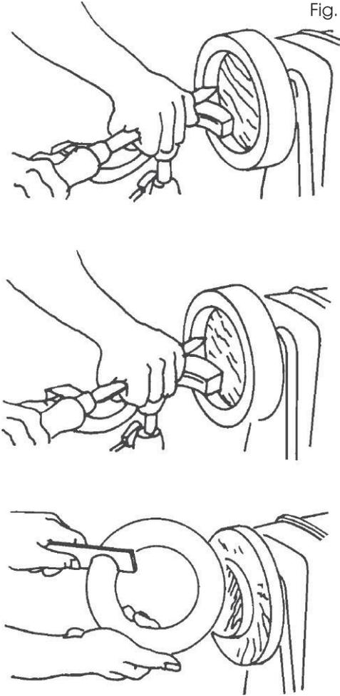
Another method of turning a ring makes use of a recessed chuck. The work stock is mounted on a screw centre and one half of the ring is formed, but the ring is not cut away from its centre. The stock is then removed and a recessed chuck, mounted on the large faceplate, is prepared to receive the ring in a tight press fit.
