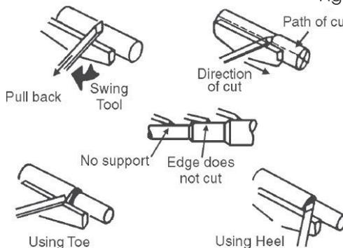
Two skews, the 1/2 and 3/4" sizes, are all that are needed for general use. Other sizes are available. This tool is nearly always used to make finished cuts, to cut vees and beads, and to square shoulders. Properly used, it produces the best finish that can be obtained with a chisel. It should not be used for scraping, as this quickly dulls it.
