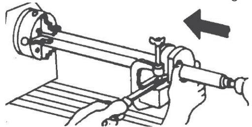
The jig uses a 1/2" gouge as the cutting tool and will produce dowels up to 11mm diameter. Make the jig from suitable hardwood stock as shown.
