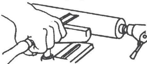
Roughing off and other heavy work requires a firm grip and solid positioning of the chisel against the rest. This is best obtained by the tool rest hand position as illustrated. The wrist is dropped down so that the heel of the hand below the little finger acts as a sliding guide against the rest. The handle hand controls chisel position.
