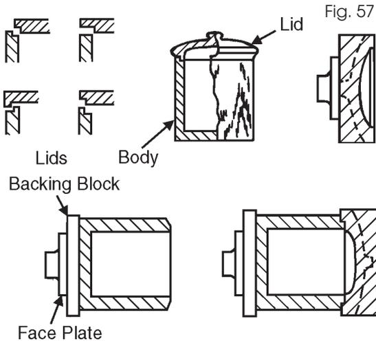
To make the 12-piece bowl, a board about 22x76x760mm, is cut into pieces about 65mm long, the saw blade being tilted 15° and the board being turned alternatively face up and face down to make the successive cuts. These 12 pieces glued together and clamped by wrapping the assembly with wire. When dry the rim thus formed is glued to a temporary circular backing which is mounted on the large faceplate.
