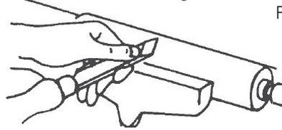
Finish cutting requires more control with less force and is better done with the palm of the tool rest hand turned up. The wrist is still held down, and the side of the index finger acts as a guide along the rest. In this position, control of the chisel is shared by both hands, the fingers of the tool rest hand being free to assist in positioning the tool.
