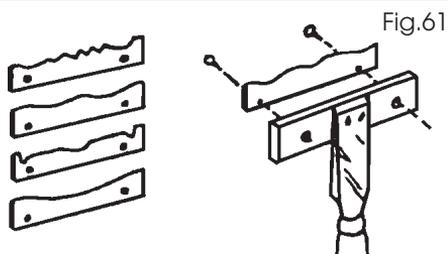
When a number of identical pieces are to be produced, all having a distinctive surface pattern, preformed tools will speed the work and assure uniformity. Patterns like those illustrated can be created by grinding thin gauge aluminium strips. A holder, like the one shown, can then be used to support any one of your prepared strips and guide it against the workpiece.
