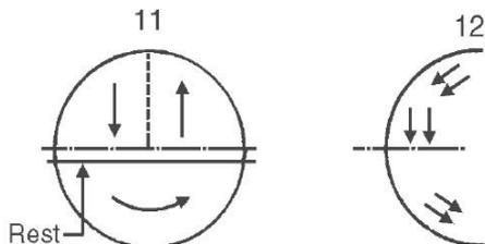
When scraping on the diameter, that portion of surface to the right of centre is moving upwards (Sketch 11). If the chisel is placed in this area, it will simply be carried up off the rest and out of your hands. All diameter scraping operations must be done at the left of centre.
