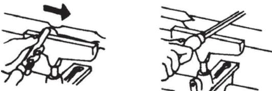
The first series of cuts should not be too deep. It is better to partially reduce the work to a cylinder along its complete length, then start a second series of cuts to reduce it to a cylinder. Once a cylinder has been formed, step the lathe up to its next fastest speed. Further reductions in size can now be carried out by cutting as deeply
