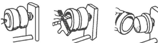
After making a recess at least 1/2 the way through the workpiece, and finishing this on the inside, remove the workpiece from the lathe. Now mount a short length of soft wood stock on the screw centre and turn this down to form a dowel that will be a tight press (not driving) fit inside the recessed end of the cylinder. Mount the cylinder on this wooden chuck, and recess the unworked end deep enough to form a perfect hole through the entire cylinder.
