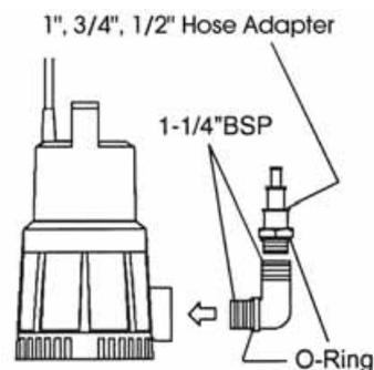
to the multi hose adapter, preferably cutting off the other two stages at the groove at the end of the 1" dia. step.
