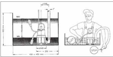
It should not normally be necessary to change the length of cable (from the clamp to the float switch), but should you do so, remember that the cable length should NEVER be so long that the float switch fails to operate and switch the pump OFF. ALWAYS check its operation before use.
