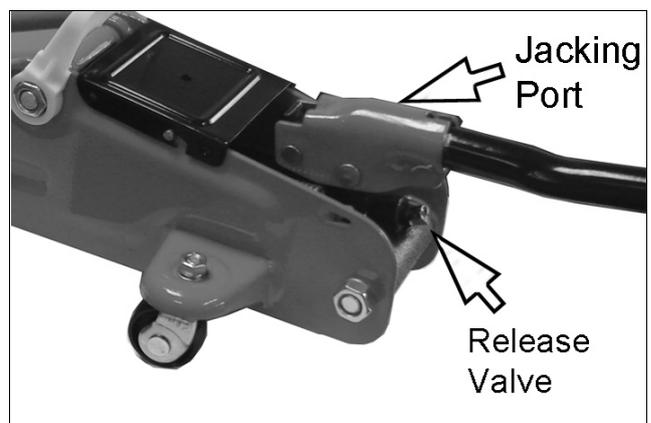
4. Place the operating lever in the jacking port and pump the operating lever so that the saddle rises to the lifting point.
