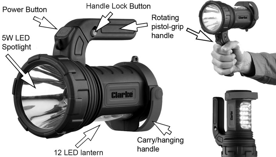
1. To operate, press the power button on the front of the handle. Press once for 100% power; again for 50% power, press again for the 12 SMD LED lantern function and once again to switch off. Squeeze the handle lock button and rotate the pistol grip handle if required.
