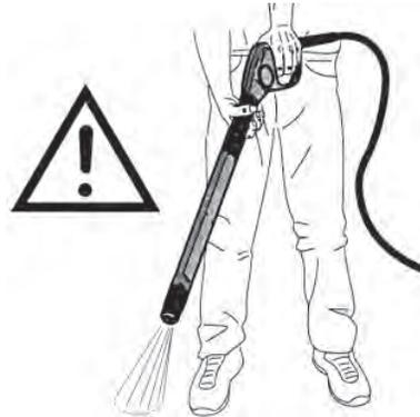
As explained above, whenever you release the trigger, the bypass valve will operate, allowing the motor to continue to run whilst water is not delivered at the nozzle. **IMPORTANT! To avoid overheating, you should never allow this condition to exist for longer than 1 minute or so.**
