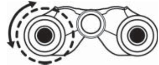
Using both eyes, rotate the focus wheel until the subject is in optimum focus.
