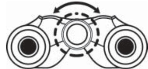
Finally adjust the zoom lever to the desired position.
