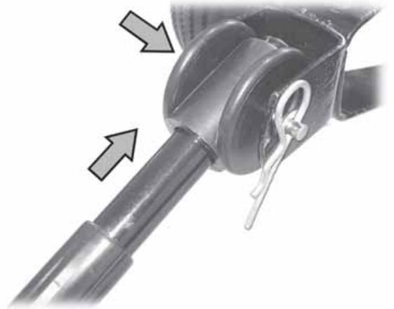
Slide the handle into the trunnion and attach the assembly to the yolk on the steering assembly as shown in fig.6. Slide the pin through the yolk and trunnion and secure with the supplied washer and 'R' clip.
