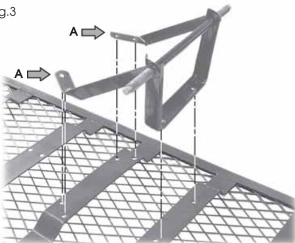
Slide the braces 'A', over the ends of the rear axle, attach the assembly to the bed using the bolts, flat washers and locknuts supplied as shown in fig.3. **NOTE:** Flat washers should be used against the nuts.
