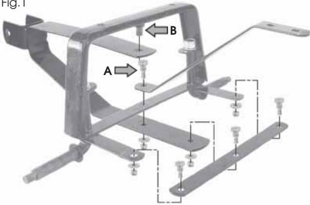
Assemble the steering linkage components as shown in fig.1. Shoulder bolts are used at all linkage points, the longest of the shoulder bolts is used at point 'A'. Secure the bracket at point 'B' using the supplied flat washer and split pin.
