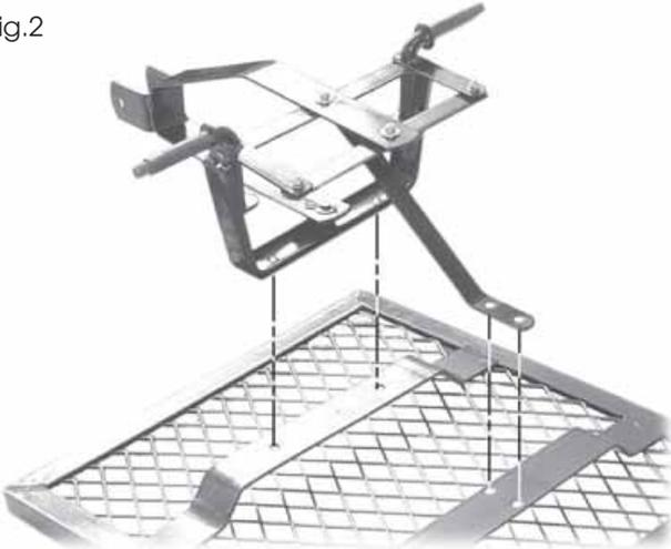
Turn the bed on its back and attach the steering linkage using the bolts, flat washers and locknuts supplied as shown in fig.2. **NOTE:** Flat washers should be used against the nuts.
