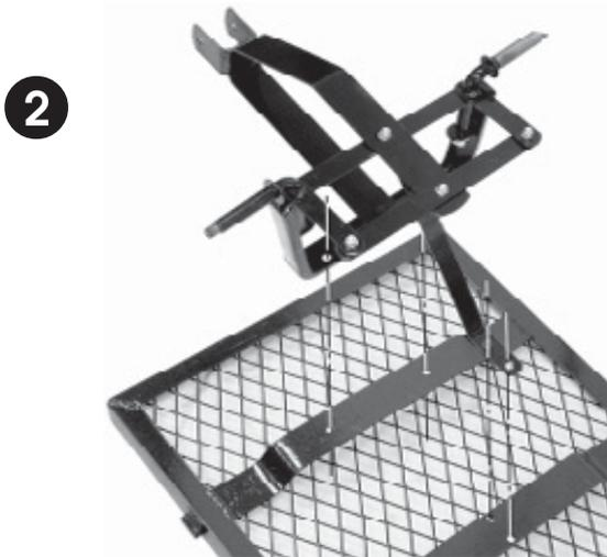
2. Turn the bed on to its back, and attach the steering linkage as shown in Fig.2, using the bolts, flat washers and locknuts supplied. The flat washers should be against the nut.
