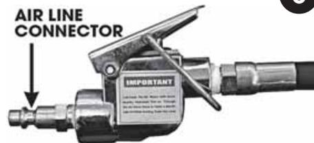
Start the compressor with the outlet pressure set to zero, then open the outlet tap.
