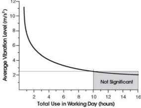
Some tools with a high vibration value, such as impact wrenches, are generally used for a few seconds at a time, therefore the cumulative time may only be in the order of a few minutes per day. Nevertheless, the cumulative effect, particularly when added to that of other hand held power tools that may be used, must always be taken into account when the total daily dose rate is determined.
