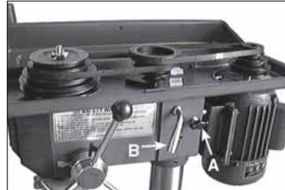
2. Lever the motor, on its bracket, away from the head, using the lever B - Fig.5, so that tension is applied to the belts.
