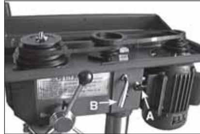
2. Lever the motor, on its bracket, away from the head, by turning lever B - Fig. 11, anticlockwise so that tension is applied to the belts.
