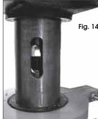
**NOTE: Morse taper drills (MT2), may also be used with this machine, and are inserted into the Quill to replace the arbour. Removal is the same as that for removing the chuck.**
