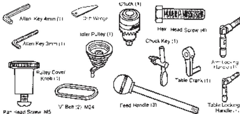
Check the parts against the above list and refer to the following diagrams. Should there be any deficiencies or damage, you should contact your CLARKE dealer immediately.
