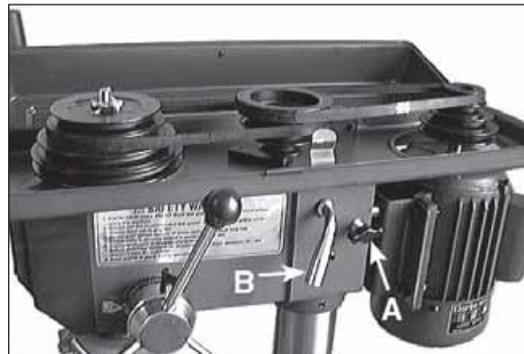
3. Consult the chart inside the belt cover (duplicated on page 12), and fit the belts in the position corresponding to spindle/drill speed required.
