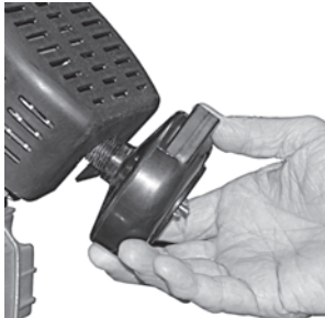
Screw on the air filter assembly fully.
